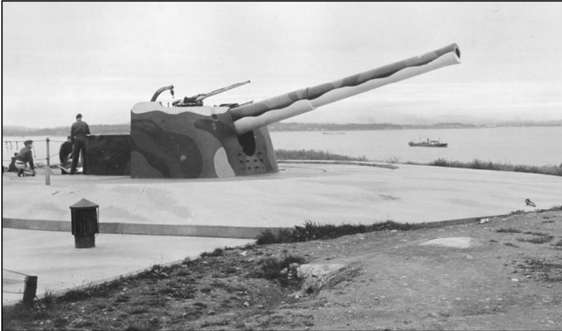
A 9.2-inch Mk 10 gun on Mk 5 Barbette Carriage, probably at Fort McNab in Halifax early in the Second World War. The 6-pounder Hotchkiss sub-calibre gun, and the auxiliary ammunition hoist can be seen above the shield. The men provide a scale for size. LAC 399220.
