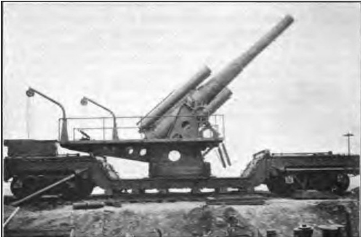
American 8-inch railway mount M1918, showing the firing platform formed by cross ties laid on H-beams. This type of mounting was installed at Prince Rupert. At Christopher Head, the gun and mounting was removed from the rail car and placed on a concrete pad. Fort Record Book.
