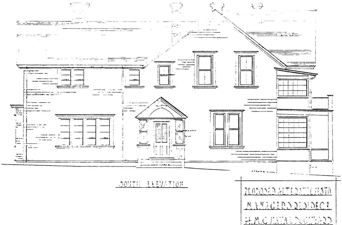
4 Building D1, side (southern) elevation, showing enlarged verandah and rear wing, new side entrance, 1931. (CFB Esquimalt.)
